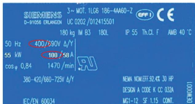
The rated operational current of the motor must be set with the  $I_e$  potentiometer according to the mains voltage and the motor connection (wye-delta). The electronic motor overload protection also refers to this set value if it is active. For the permissible settings referred to the required motor overload trip class, refer to chapter Motor current settings (Page 113).
