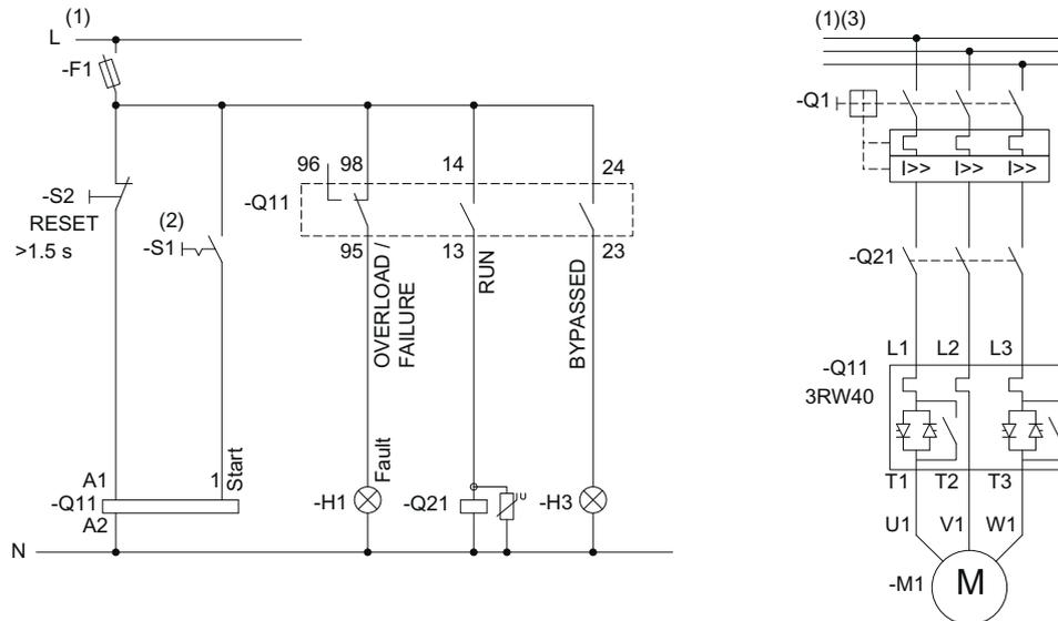
Figure 15-15 Wiring of the 3RW40 2 to 3RW40 4 control circuit and the 3RW40 2 to 3RW40 7 main circuit
