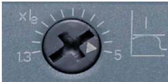
The current limiting value is set with the  $xI_e$  potentiometer to the maximum required starting current as a factor of the set rated motor current ( $I_e$ ).
