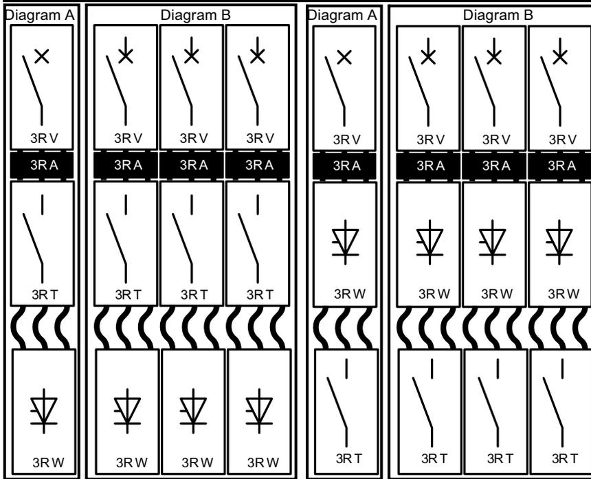
Assembly of 3RW with 3RV2 motor starter protector and 3RT line contactor with cable. The minimum clearance between the 3RV and 3RT corresponds to the minimum clearance (b/c) in the diagram of clearances from other devices.
