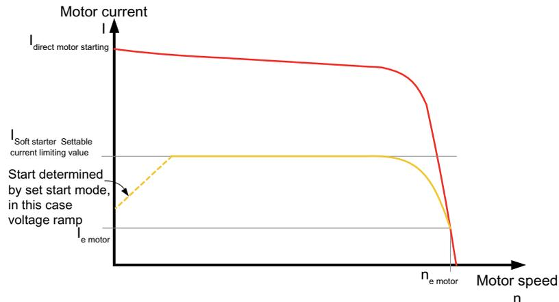
The SIRIUS 3RW40 soft starter measures the phase current (motor current) continuously with the help of integrated current transformers.
