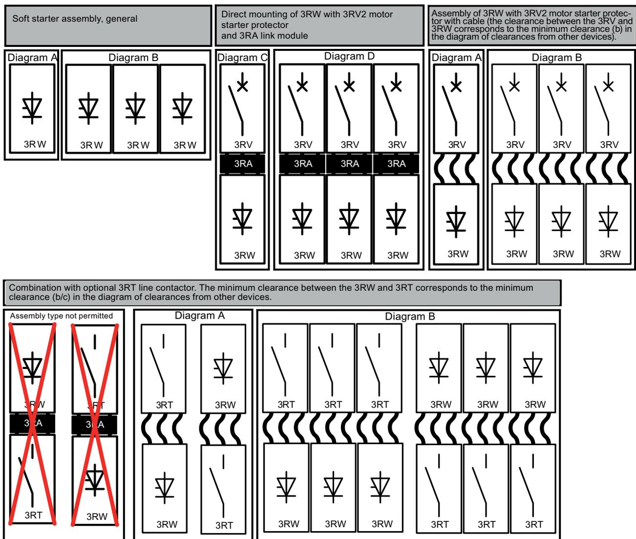
Assembly of 3RW with 3RV2 motor starter protector, 3RA link module, cable, and 3RT line contactor. The minimum clearance between the 3RW, 3RV, and 3RT corresponds to the minimum clearance (b/c) in the diagram of clearances from other devices.
