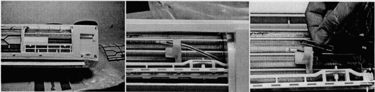
With this modification you tell to electronics that the room temperature is aprox. 7 degrees warmer then actually is. This is shifting for 6, 5 or 7 degrees approximately. If you put 16 degrees heating on remote controller, following will happen:
