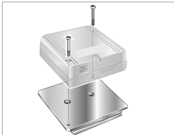
Figure 12: Attaching MC35i Terminal to a top-hat rail
